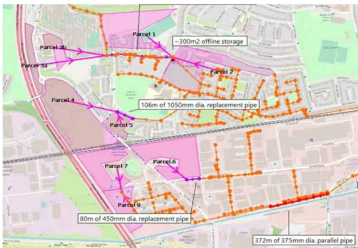
Figure 8-13 Uisce Éireann Upgrade works map
